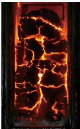
Large scale 250kg test coke oven
